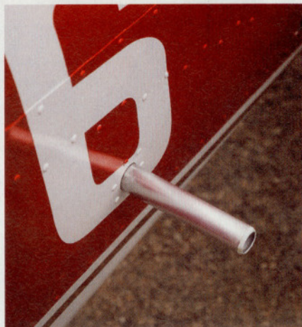
THE EXTENDABLE tail-pull handle (left) facilitates aircraft ground handling, and the custom exhaust fairing (right) reduces drag and enhances engine cooling.
