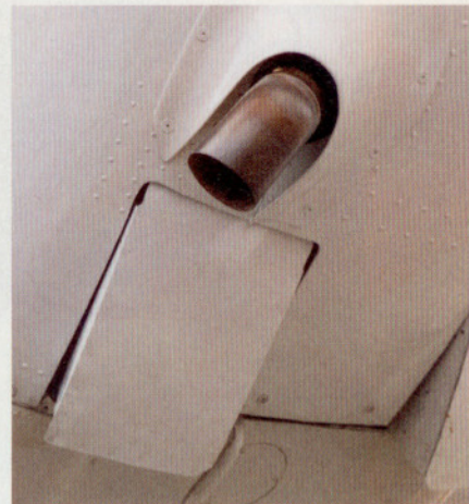
THE EXTENDABLE tail-pull handle (left) facilitates aircraft ground handling, and the custom exhaust fairing (right) reduces drag and enhances engine cooling.
